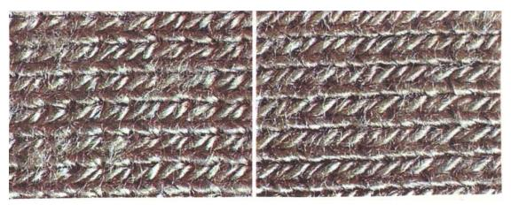
Not singed: Finished fabric after 5 washing cycles Singed (Dornier): Finished fabric after 5 washing cycles
